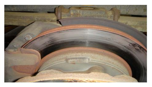
The rotor shown below exhibits severe brake pad material transfer and is a good indicator that the brake caliper assembly at this wheel end had experienced brake drag that may be related to the safety defect. The excessive amount of brake pad material transferred on to the rotor would be considered collateral damage and will require the replacement of the rotor. The associated cost is covered by the interim repair procedure if a caliper failure has occurred.
