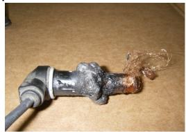
ABS sensors experiencing heat damage that may be related to the safety recall have stopped functioning at various speeds and may have intermittent or complete loss of functionality and associated fault codes.
