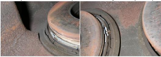
Heat damaged ABS system wheel speed sensors
