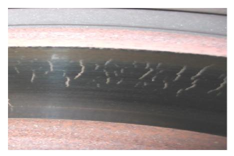
The existence of cracked rotors as described above, and without any other evidence (see additional items described below), would not justify a caliper replacement per the interim letter – neither would the replacement of the rotor qualify for a goodwill policy replacement. A replacement of the rotor under these conditions would be the responsibility of the customer.
