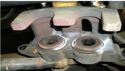
Cracked piston dust seal/boot (white residue may also be present)
