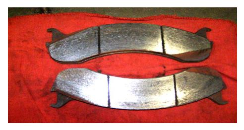
The brake pad shown below exhibits the rough/damaged surface typically associated with material transfer from the pad to the rotor due to excessive heat. The corresponding rotor will most likely exhibit corresponding material deposits from these pads. Replacement of a brake pad in this condition is considered collateral damage and is covered by the interim repair procedure.
